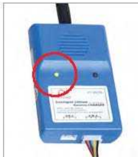
Completed (LED: Green)
